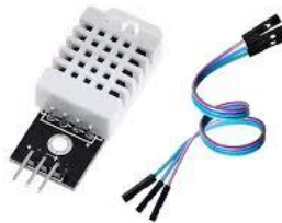
Gambar 1. Sensor DHT22
